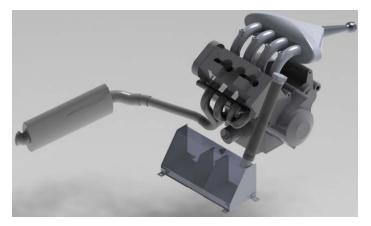
been made to the intake manifold by adding bell mouths and using flow simulation. By changing the intake's mounting orientation, the center of gravity for the car has been lowered. The final version of the intake will be printed by our *Go Engineer* sponsor using ULTEM 1010 resin. The exhaust runners have also been rerouted for weight reduction and easier access to the oil filter. Additionally, the fuel tank has been redesigned to prevent fuel starvation.
