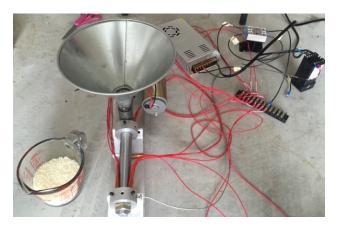
in unison, with a thermocouple measuring the temperature. A solid-state relay is attached to the thermocouple, giving users the ability to set a desired temperature. The melted plastic will then be pushed through a nozzle by a rotating screw, which is attached to a motor. This is the extrusion process, which will shape the material into a long filament that can be spooled.
