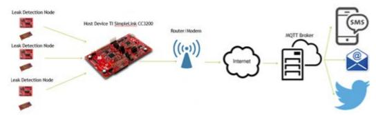
Unchecked, a leak can quickly turn into large amounts of water gushing into a home or business damaging the structure, electrical wiring, or belongings. Our goal is to create a water leak detection system that will alert users of
