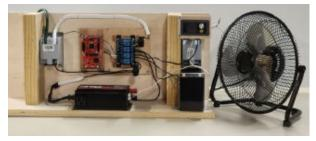
throughout the day. The Microgrid Load-Shedding Controller (MLSC) is the device we created to address these issues. The goal of the MLSC is to reduce the energy demand on the grid. Our device manages a battery system to supplement power during high-demand hours. Our scaled-down model is designed to supply power for a single household appliance, such as an air conditioner, electric range, or central heating unit.
