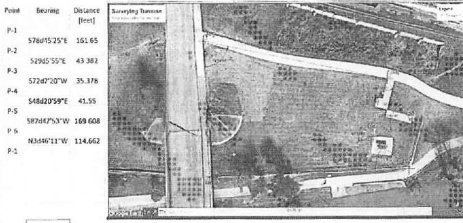
Figure 7 – Completing the Traverse in Auto-Cad knowing the local coordinates of traverse corners
