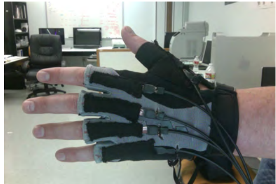
Fig. 4. Bend Sensors mounted on a glove
