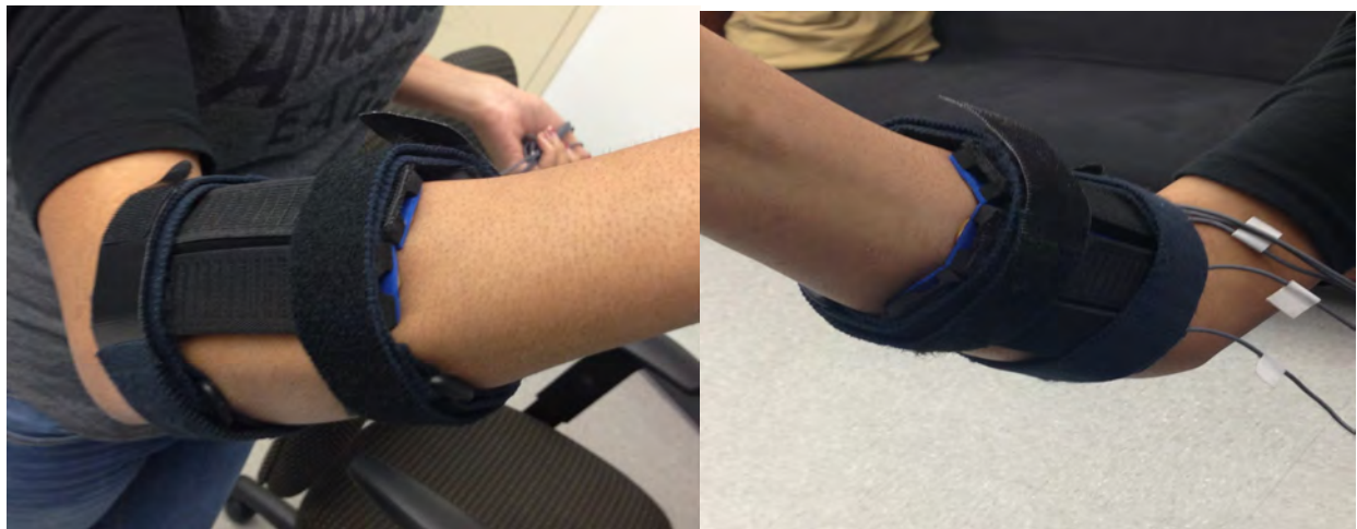
Fig. 5. Modified Bioflex Sensors (placed along the upper forearm and upper underarm)
