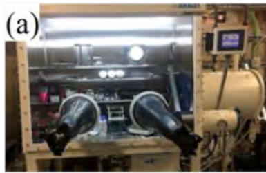
Equipment for battery research (Dr. Choi's lab): (a) Glove Box; (b) Electrochemical Workstation (GAMRY); (c) Battery Tester (MACCOR, 32 channels); (d) Battery tester with temperature control oven; (e) 4-Probe Station.
