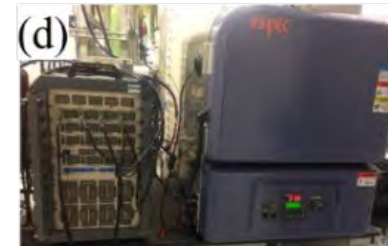
Equipment for battery research (Dr. Choi's lab): (a) Glove Box; (b) Electrochemical Workstation (GAMRY); (c) Battery Tester (MACCOR, 32 channels); (d) Battery tester with temperature control oven; (e) 4-Probe Station.
