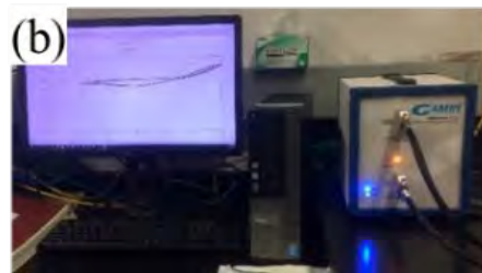
Equipment for battery research (Dr. Choi's lab): (a) Glove Box; (b) Electrochemical Workstation (GAMRY); (c) Battery Tester (MACCOR, 32 channels); (d) Battery tester with temperature control oven; (e) 4-Probe Station.
