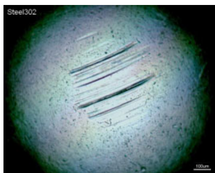
Figure 9. 302 steel ball surface after friction with TPV + ceramic at 1.0 N.
