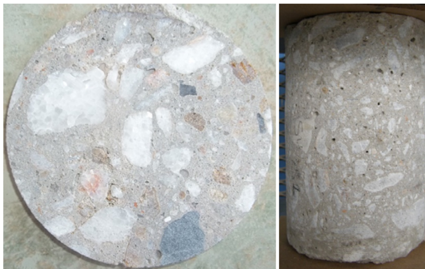
Fig. 2. Distribution of aggregates in concrete specimens: from top (left) and from the side (right).
