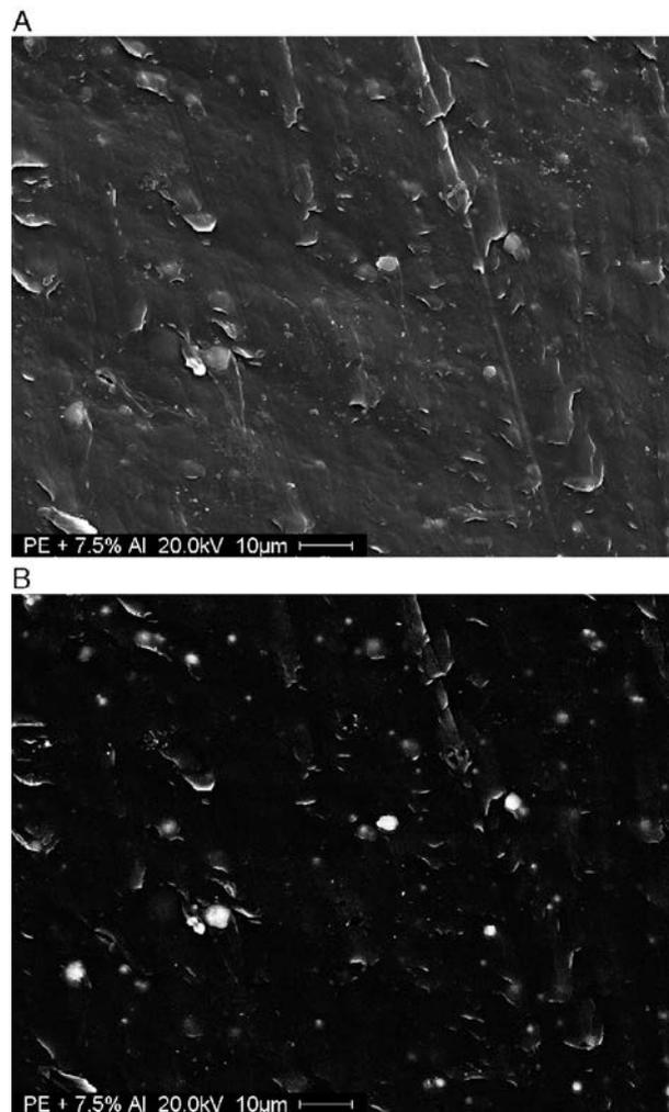
Fig. 1. A) Secondary electron image of PE+7.5 wt.% Al powder. B) Backscattered electron image of PE+7.5 wt.% Al powder.
