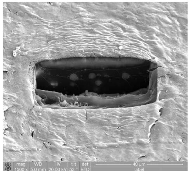
Fig. 4. FIB cross-section after low current beam cleaning.
