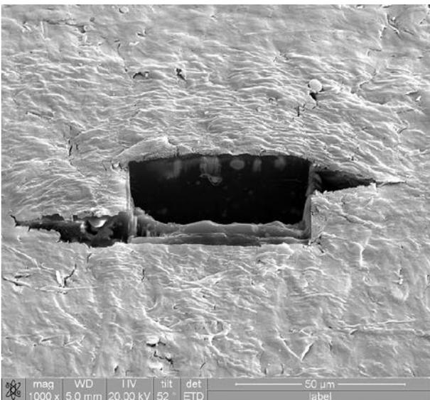
Fig. 3. FIB cross-sectioned box of PE+10% Al microhybrid.
