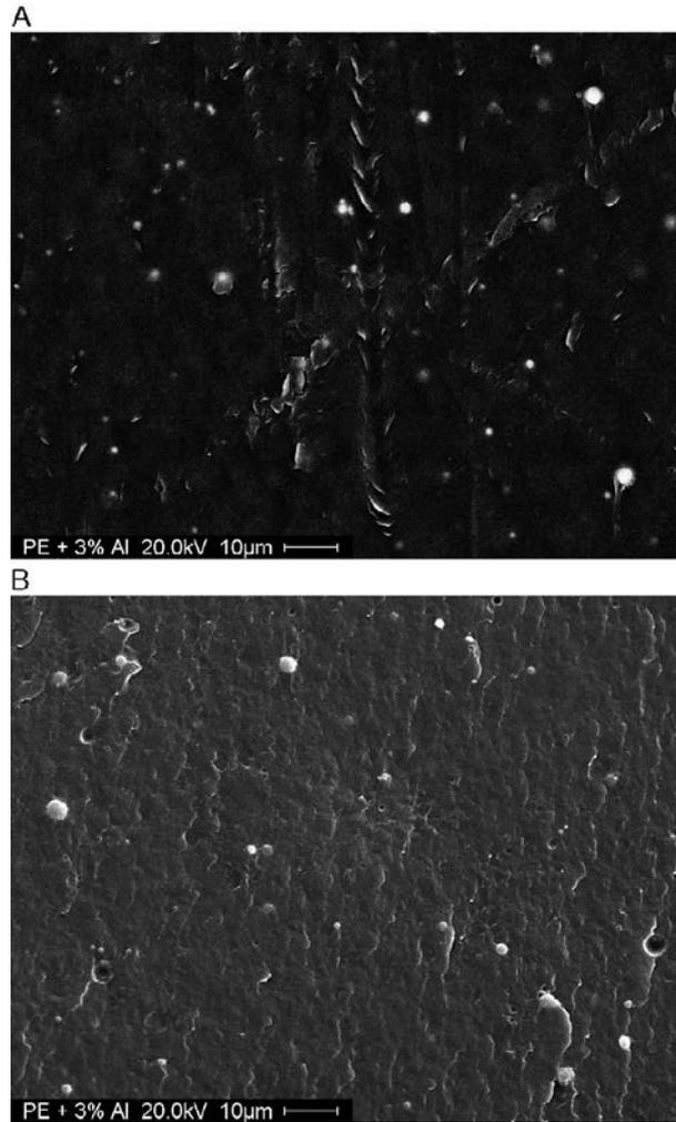
Fig. 2. A) SEM image of the composite surface of PE+3 wt.% Al powder. B) SEM image of the composite cross-section of PE+3 wt.% Al powder.
