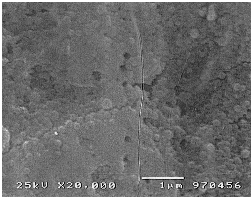
Fig. 6. SEM micrograph of the sample as in Fig. 5 but thermally treated in air at 900°C.
