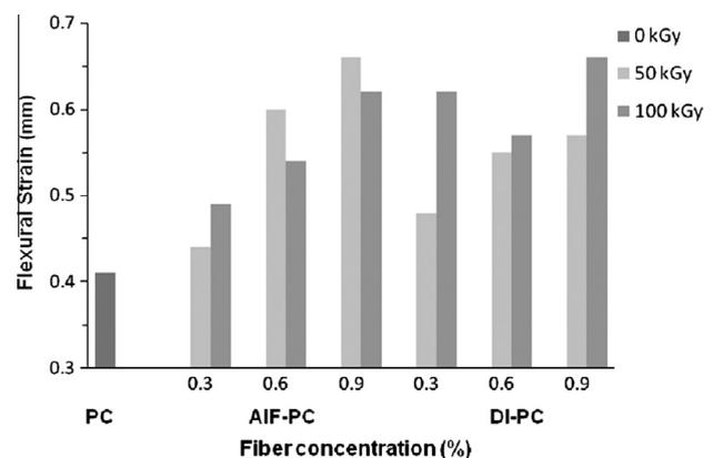
Fig. 6. Flexural strain of polymer concretes with luffa fibers.
