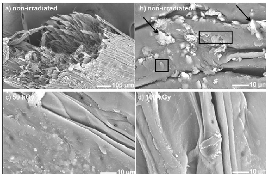
Fig. 9. SEM images of non-irradiated and irradiated luffa fibers.
