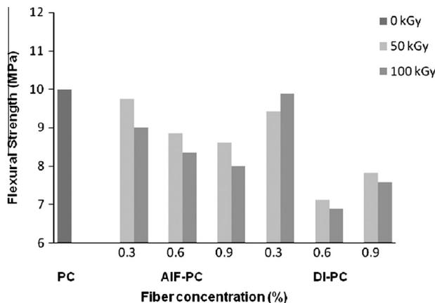
Fig. 5. Flexural strength of polymer concrete.
