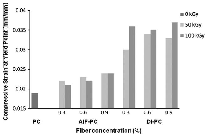
Fig. 4. Compressive strain at yield point of polymer concrete.
