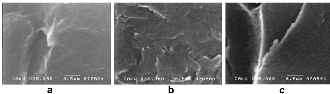
Fig. 3. SEM images of polyester resin: (a) non-irradiated; (b) irradiated at 50 kGy; and (c) irradiated at 100 kGy.
