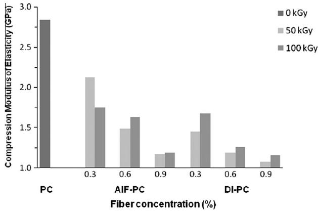
Fig. 7. Compression modulus of elasticity of polymer concretes.
