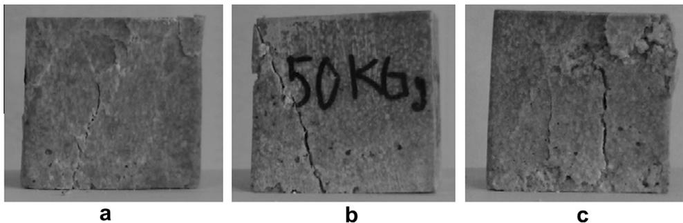
Fig. 2. AIF-polymer concrete specimens after testing: (a) non-irradiated, (b) irradiated at 50 kGy, and (c) irradiated at 100 kGy.
