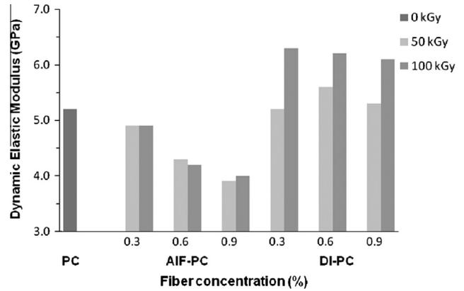
Fig. 8. Dynamic elastic modulus of polymer concretes with luffa fibers.
