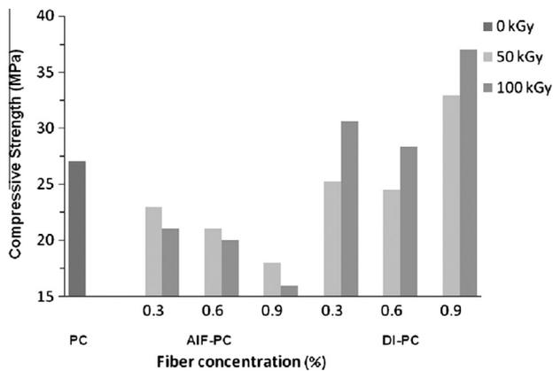
Fig. 1. Compressive strength of polymer concrete.
