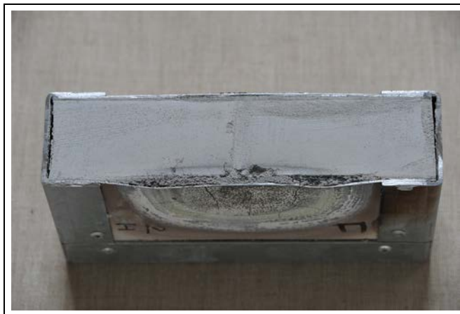
Figure 3. A 50-mm-thick sample imitating a fire door element after solar irradiation maintaining 950°C for 1 h; a cross section (a side view similar to that in Figure 2).
