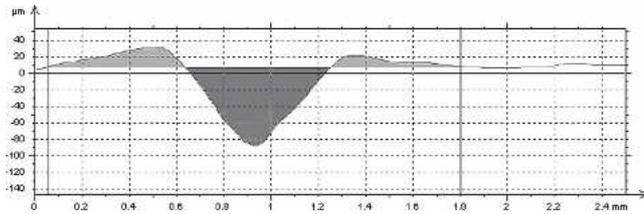
FIG. 3. A profile of a scratch trace on a PTFE surface. Other details are as in Fig. 1.
