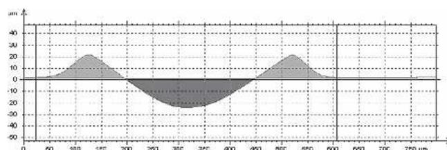
FIG. 1. A profile of a scratch trace on a PES surface for the applied load of 15.0 N. The profile is perpendicular to the side and goes through the center of the groove.
