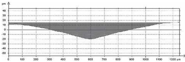
FIG. 2. A profile of a scratch trace on a LDPE surface. Other details are as in Fig. 1.
