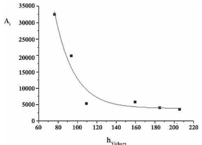
FIG. 5. Groove area  $A_i$  as a function of  $h_{\text{Vickers}}$ .
