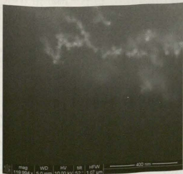
Fig. 4. FIB cross section of the 0.30 wt% PS + gold nanoparticles hybrid.
