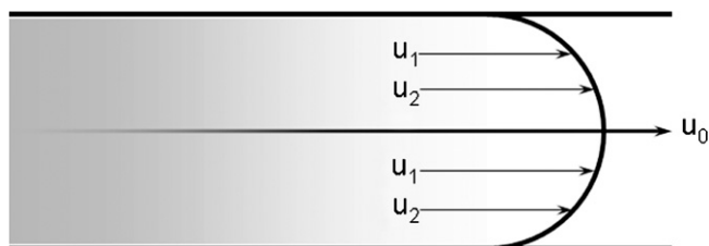
Fig. 1. Laminar flow at velocity u in a cylindrical conduit.
