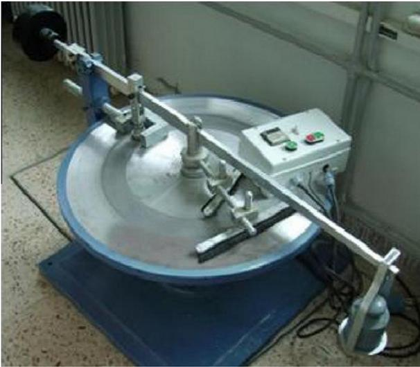
Fig. 2. Abrasive wear test apparatus.
