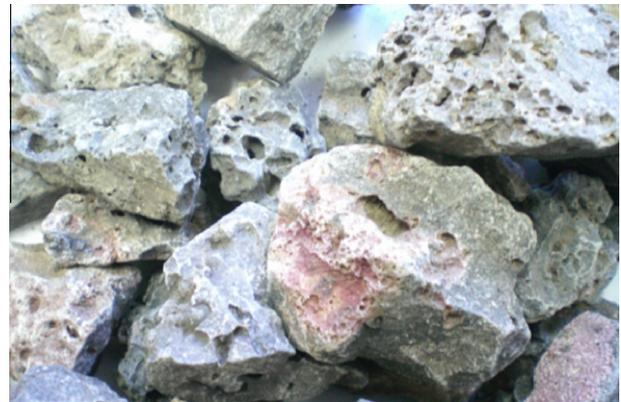
**Fig. 1.** Ferrochromium slag aggregates.
