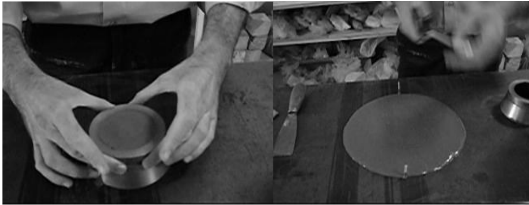
Figure-1. Slump flow test on SCM mortars
