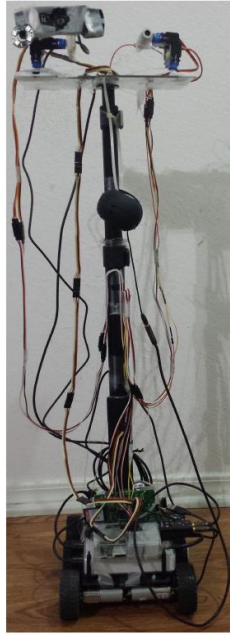
Figure 1: A Sample CARE Device. This device is deployed at the worker's location. A camera provides visuals, and a microphone and speaker provide audio. The device includes a wheeled platform for mobility.
