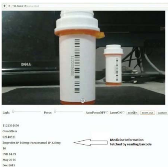
Figure 4: Remote nurse reading 2D DataMatrix barcode on the medicine bottles; Medicine information is shown in bottom half of the controlboard
