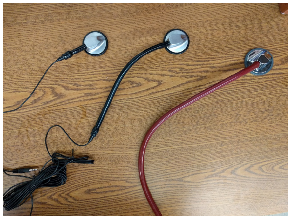
Fig. 4. Different lengths of stethoscope tubes used for testing the impact of the length on the quality of heart sounds.
