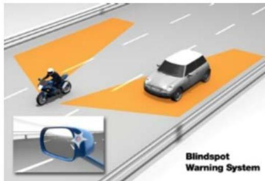
Figure 1: Diagram of Sensor Detection Area
